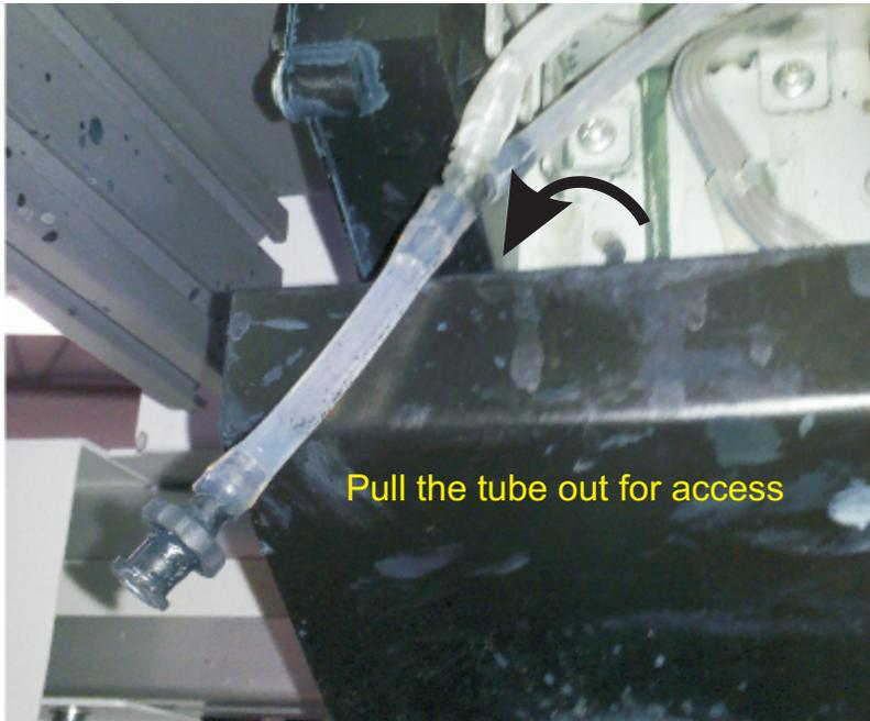
The tube has a connector that can connect directly to your syringe. You can apply flushing solution to your capping station and then use the syringe to draw the flush through the capping station.
